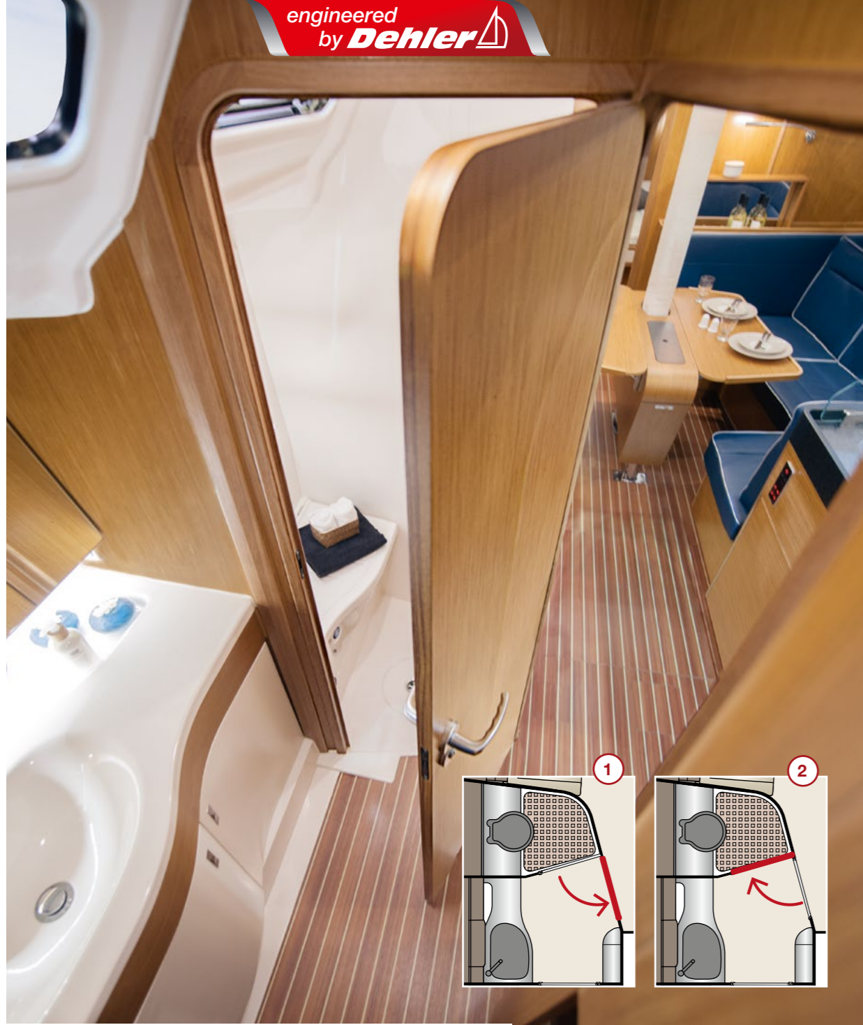
The Dehler Uni Door Concept creates two different room layouts.
